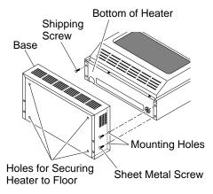
Figure 18 - Attaching Heater to Hearth Base
